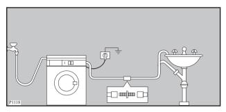
For a correct functioning of the machine the drain hose must remain hooked on the proper support piece situated on the top part of the back side of the appliance.
